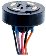
K171H Locking Type Receptacle, 7-Pin, C136.41 Compliant, 12" lead
